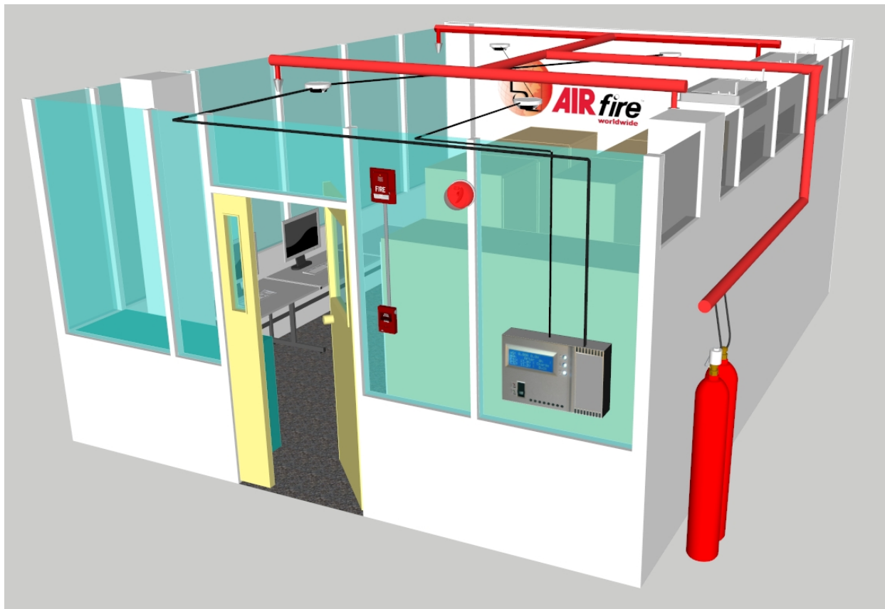
Figure 83 - Gas suppression system basic layout
