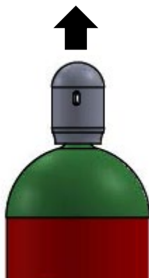
Figure 48 - Removing cylinder transport cap
